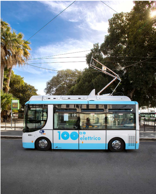
▶ In motion charging trolleybus (Cagliari)
