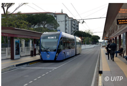
➤ Infrastructure for in motion charging
