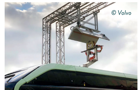
➤ Roof-mounted pantograph charging
