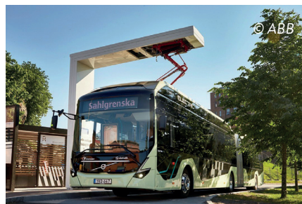
➤ Infrastructure-mounted pantograph charging
