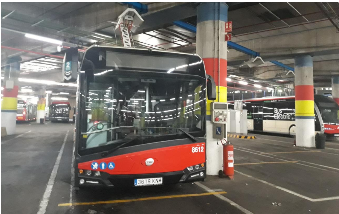
► Depot charging with pantograph solution (50 kW). Source: TMB Barcelona
