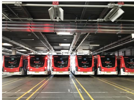
► Pantograph-based charging on racks a) openair-rack infrastructure at Harlem depot (Transdev NL); b) indoor-rack on ceiling, at Eindhoven depot (Hermes/Transdev). Source: A. Abdulah, UITP
