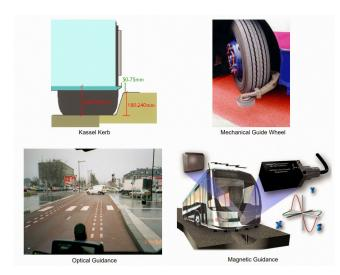
Figure 24. Examples of precision docking systems
