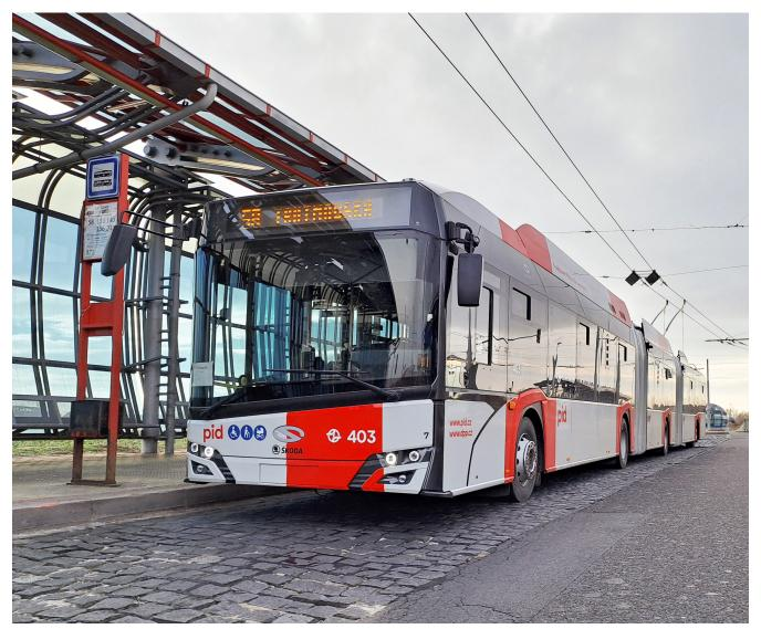
*Figure 1.* In-Motion Charging trolleybus BRT in Prague © DPP
