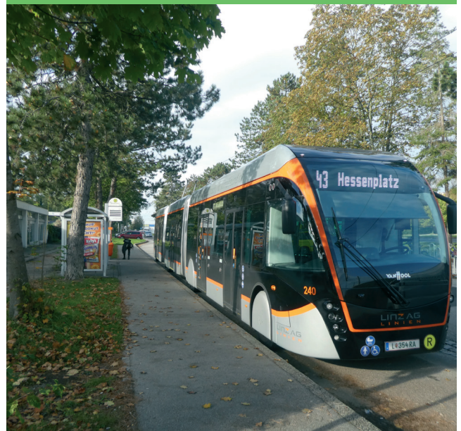
▶ A state-of-the-art, 24 metre long double-articulated IMC bus in Linz, Austria is an efficient solution to capacity with a small battery of only 60kWh.
