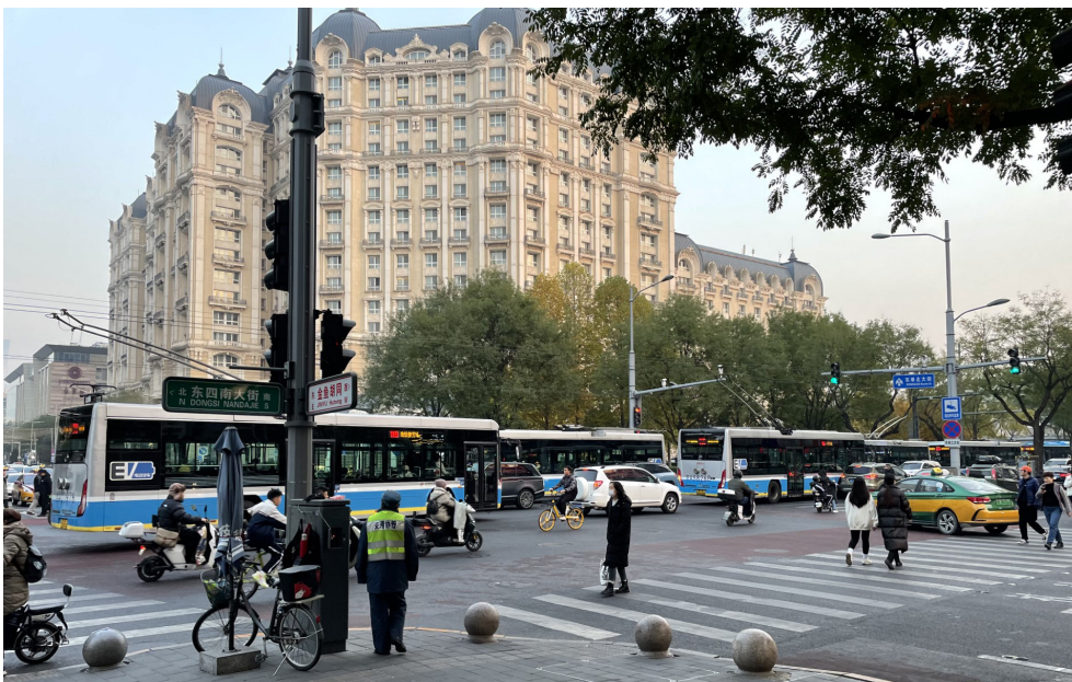
► Main urban corridor in Beijing, China, illustrating the ‘charging road’ concept: Overlaying IMC trolleybus routes operate at high frequency in mixed traffic on a single set of wires, allowing for charging and overtaking with off-wire operation.
