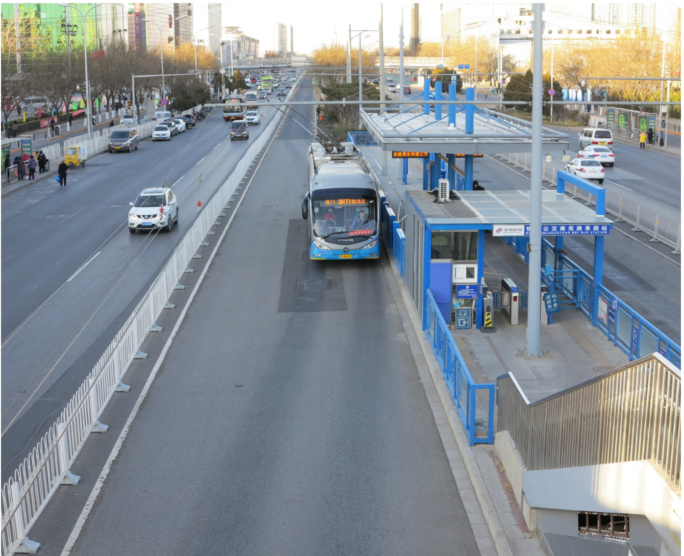
► Station on an eBRT corridor operating with IMC trolleybuses in Beijing, China.
