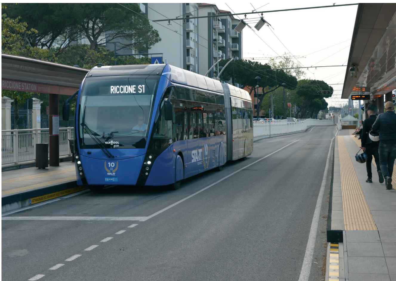
▶ In Rimini, Italy, a new eBRT (electric BRT) route of 9.8km opened in 2021, running almost exclusively on dedicated right-of-way. Route extensions are currently being planned.
