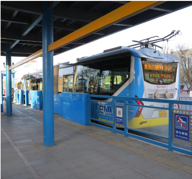
▶ An 18m IMC trolleybus operating in eBRT service in Beijing, China. Beijing has 2 out of 3 BRT routes electrified with IMC technology.
