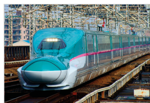
Series E5 Shinkansen operating at Japan's maximum rail speed 320km/h.
