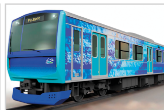
"HYBARI (Hydrogen-Hybrid Advanced Rail vehicle for Innovation)" was tested as a hybrid (fuel cell) test train. Scheduled to debut in 2022.
