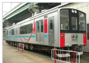
"NE-Train (New Energy Train)," the world's first hybrid train, developed in 2003.
