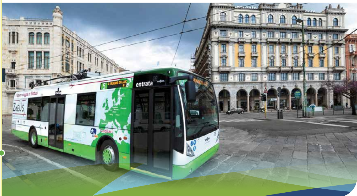
Battery trolleybus driving on battery-mode disconnected from overhead wires in Cagliari (Source: Consorzio Trasporti e Mobilità S.p.A.)
