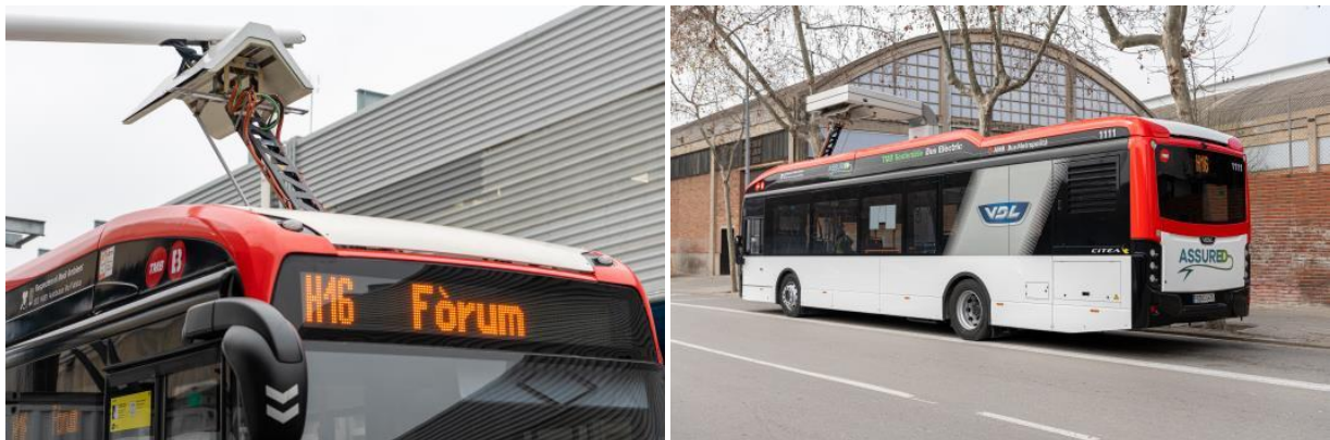
Pantograph charging of a test bus at the depot and at an H16 stop
